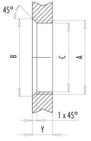
Installation direction: o-ring sits on chamfer.
